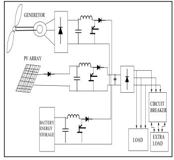
Fig. 1: Configuration of Hybrid Energy System
