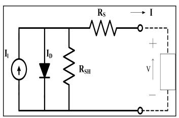
Figure 3: Equivalent circuit of PV Module
