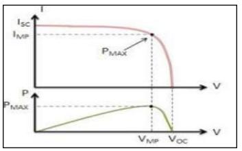
Fig. 4: Output characteristics of PV Array
