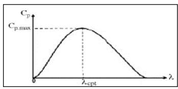
Fig. 2: Power coefficient vs Tip Speed Ratio
