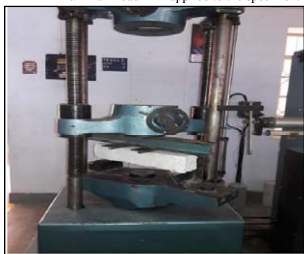
Fig.9: Testing setup for flexural strength
