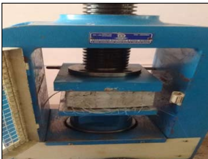
Fig 8: Compressive test of light emitting concrete
