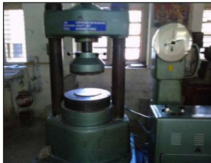
Fig. 4 : Compression strength testing machine
